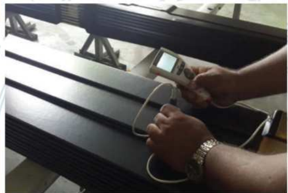
Epoxy Thickness Test
