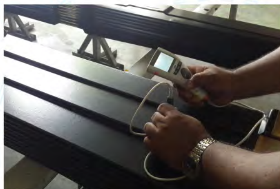
Epoxy Thickness Test
